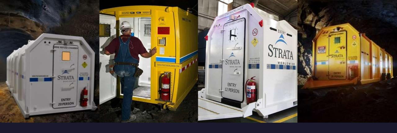
We build complete emergency refuge shelters with industrial-level safety systems built for the critical purpose of providing a safe to breathe, isolated atmosphere when the breathing air in the working section has become compromised. These products area ideal for incidents such as a fire outbreak, ventilation failure, sudden release of toxic gas or a gas related explosion. Our chambers are easily tailored to meet local, federal and industry regulations, including HVAC system.
